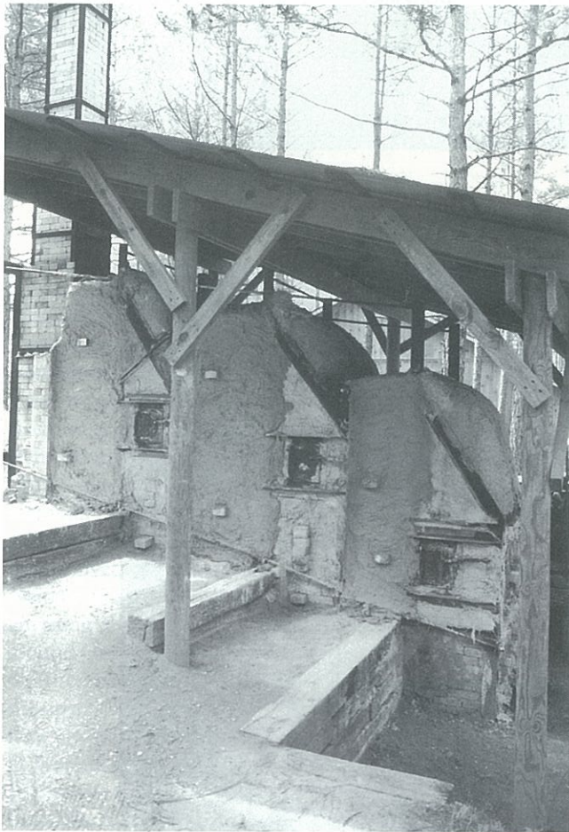
Ready to fire: all three chambers are loaded, then the doors are bricked and sealed with a mixture of clay and sand.
